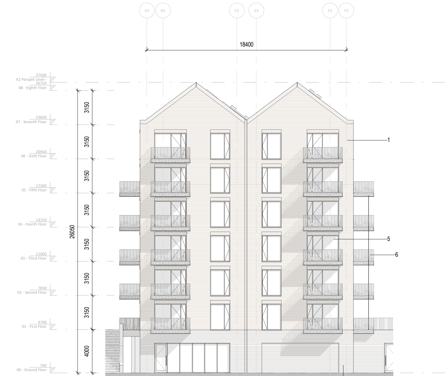
4 A3_South West Elevation 1:200
